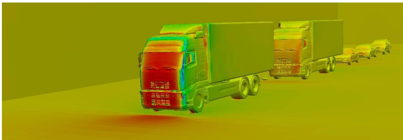
Figure 101: Platoon configuration used for CFD tests in SARTRE project [94]
